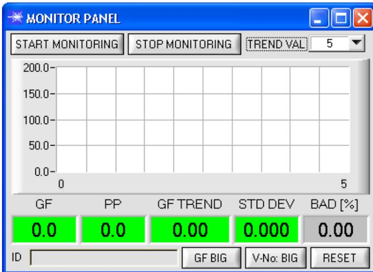
**START MONITORING** starts gloss factor monitoring. After every trigger event the sensor automatically sends the current gloss factor to the PC. This gloss factor is visualised in the GF display and in the graph. Under **TREND VAL** you can set how many of the last data frames are shown in the graphic display. The **GF TREND** display shows the gloss factor mean value that is calculated from the values that are displayed in the graph.
