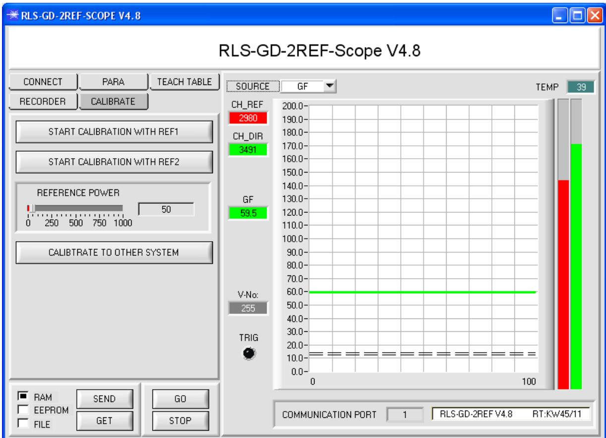
After a click on **START CALIBRATION WITH REF1** the software will ask you to place a reference calibration surface before the sensor. After confirmation with **YES** a suitable **POWER** value will be set such that channel **CH\_DIR** or **CH\_REF** lies in the upper third of its dynamic range.
