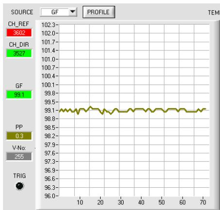
Pressing the **PROFILE** button shows the internally recorded buffer that is used for evaluation on the graphic display. The display furthermore shows **PP**, the peak-to-peak value.
