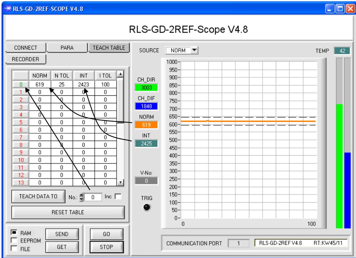
Now press the **SEND** button to inform the sensor about the taught vector. Then activate the **GO** mode again. When the sensor recognises a row vector, the corresponding row number is visualised on the software interface under **V-No.:**. A value of 255 means that none of the taught vectors were recognised.
