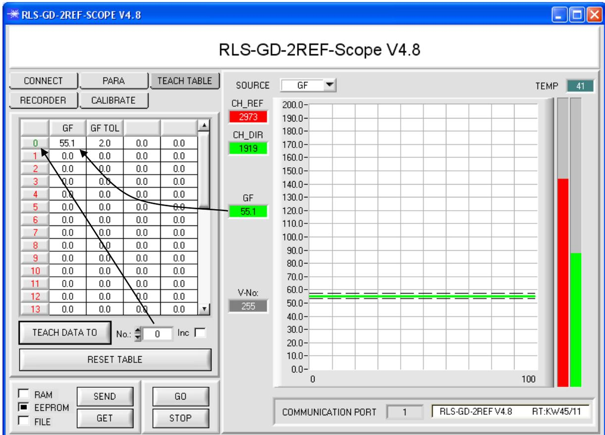
Now press the **SEND** button to inform the sensor about the taught vector. Then activate the **GO** mode again. When the sensor recognises a row vector, the corresponding row number is visualised on the software interface under **V-No.:**. A value of 255 means that none of the taught vectors were recognised.
